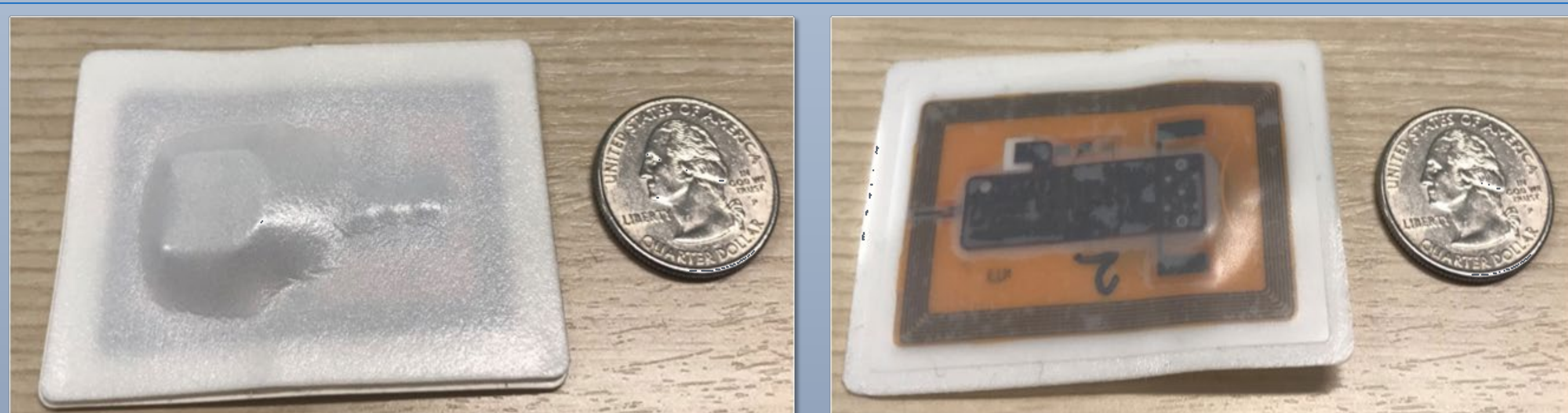
Figure 5: PATCH prototype- flex circuit encased between two layers of adhesive. (Left) PATCH side exposed to environment; (Right) PATCH side in contact with skin
